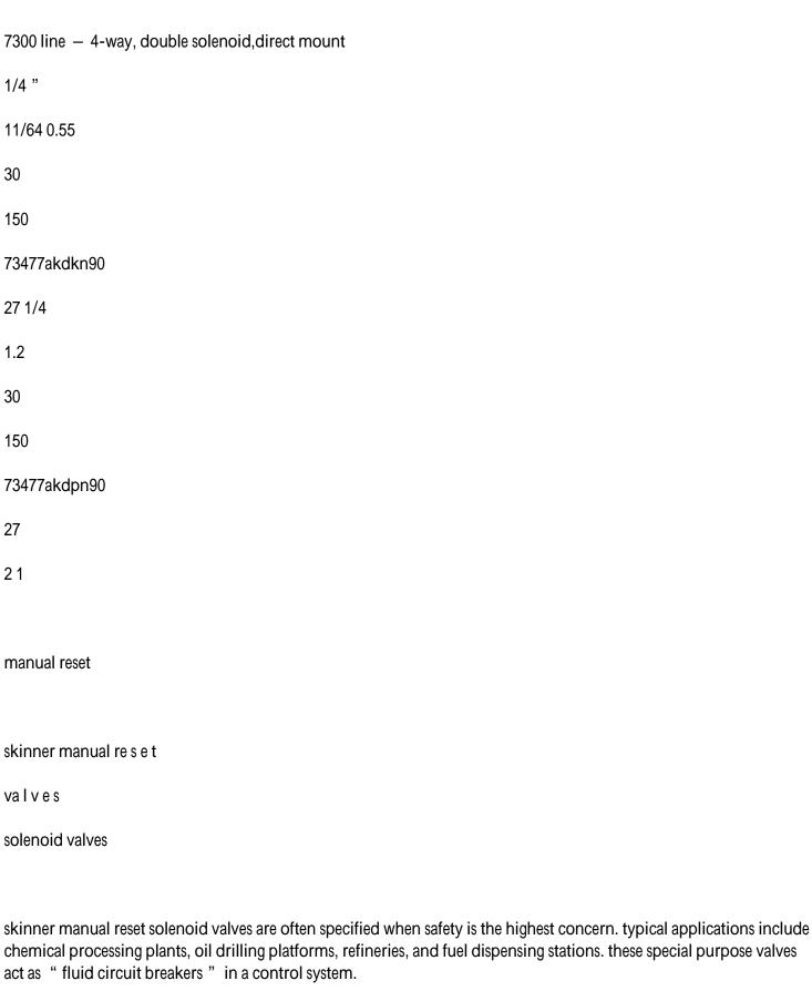
skinner manual reset valves are available in either electrically tripped or no-voltage-release models. to operate an electrically tripped or no-voltage-release models.
